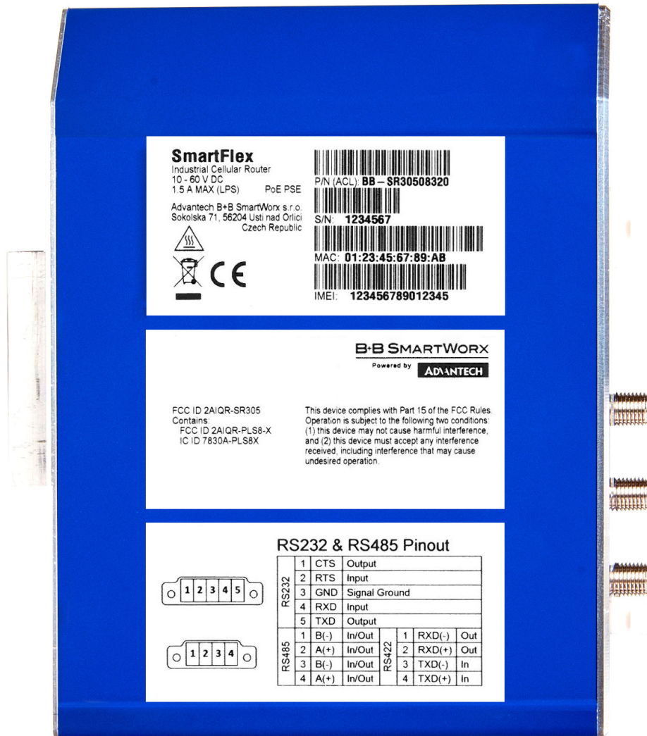
Figure 7: Example of labels on bottom of v3 metal router – from top: Product label, Certifications label (optional) and Interface label (optional).
